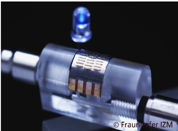
Fig. 2. Micro fuel cell powering a LED, bended configuration.
